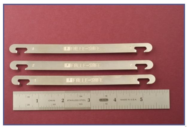
Figure 16. Falle-Safe torque tools (front; from bottom: 1, 2, 3).
