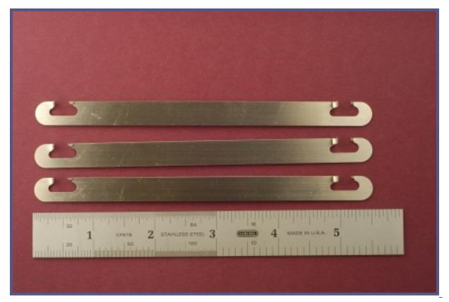
Figure 17. Falle-Safe torque tools (back; from bottom: 1, 2, 3).
