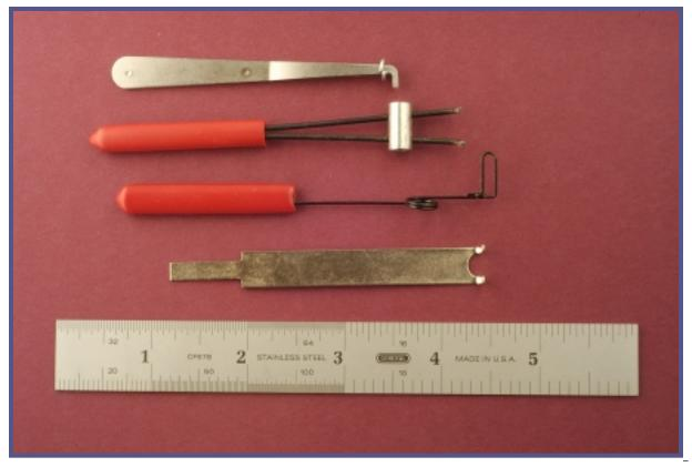
Figure 21. Other torque tools (from bottom: LAB 2-prong, HPC Feather, HPC Variable, Tweezer).
