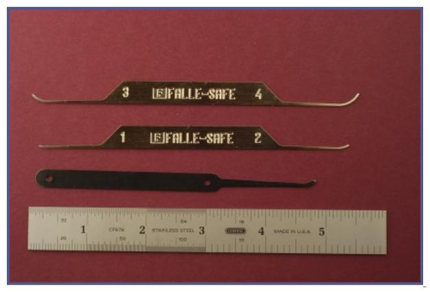
Figure 7. Falle-Safe "thin curve" picks (from bottom: 1/2, 3/4).
