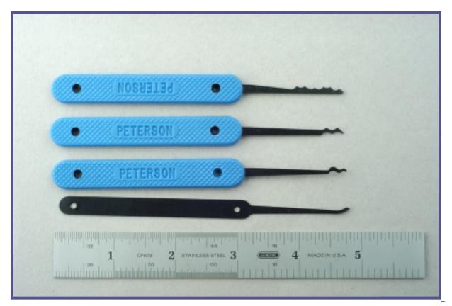
Figure 10. Peterson "rake" picks (from bottom: "Double", "Triple", "Ripple").
