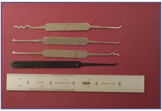
Figure 1. LAB picks (half diamond, rakes).
