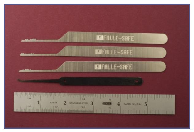
Figure 8. Falle-Safe "rake" picks.
