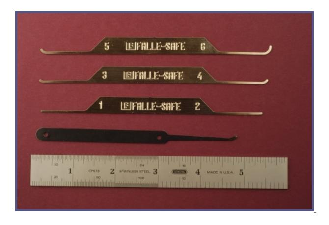
Figure 6. Falle-Safe "progressive curve" picks (from bottom: 1/2, 3/4, 5/6).
